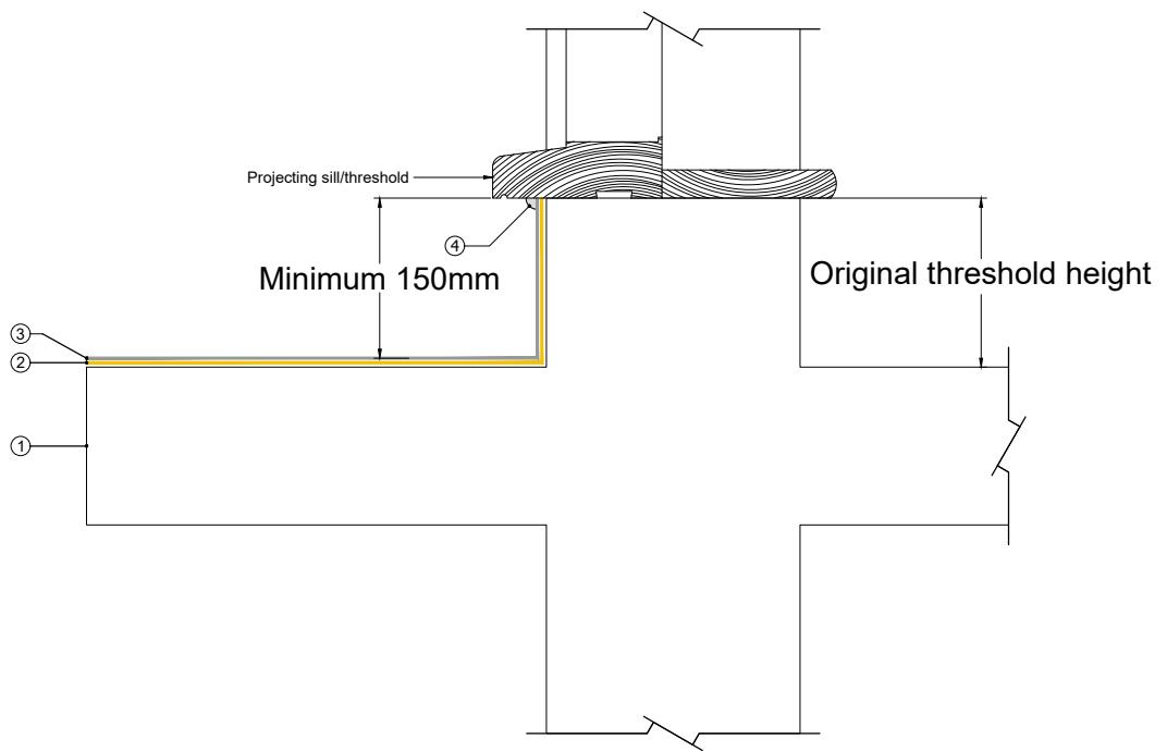
**Upstand Lead Flashing**
